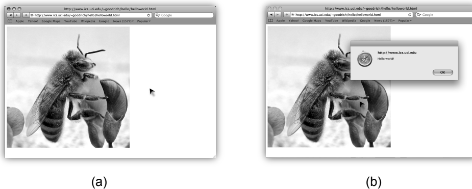
Figure 7.9: A mouse-over event that triggers a Javascript function, using the Apple Safari browser: (a) Before the mouse-over event. (b) After the mouse-over event.
