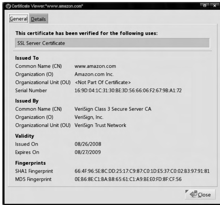
Figure 7.5: A web server certificate as displayed by Firefox. The fields of the certificate include the name of the organization owning the web site, the domain name of the website, the name of the CA that issued the certificate, the expiration date, and cryptographic parameters.
